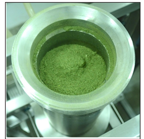
EXTRACTION VESSEL is packed full of dried cannabis that has been very finely grated through a stainless steel screen. The vessel, manufactured by machinists employed by Critical Solutions, is six inches in diameter and four feet deep. It holds 20 liters — typically, six pounds of ground cannabis, which will yield about three liters of essential oil.
