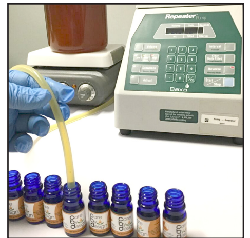
PERISTALTIC PUMP releases uniform amounts of cannabinoid-rich mixture through tube to fill sublingual spray bottles. Beaker at left contains essential oil with one of five CBD-to-THC ratios, mixed with coconut oil. Magnetic stir plate keeps the blend well-mixed throughout the process.
